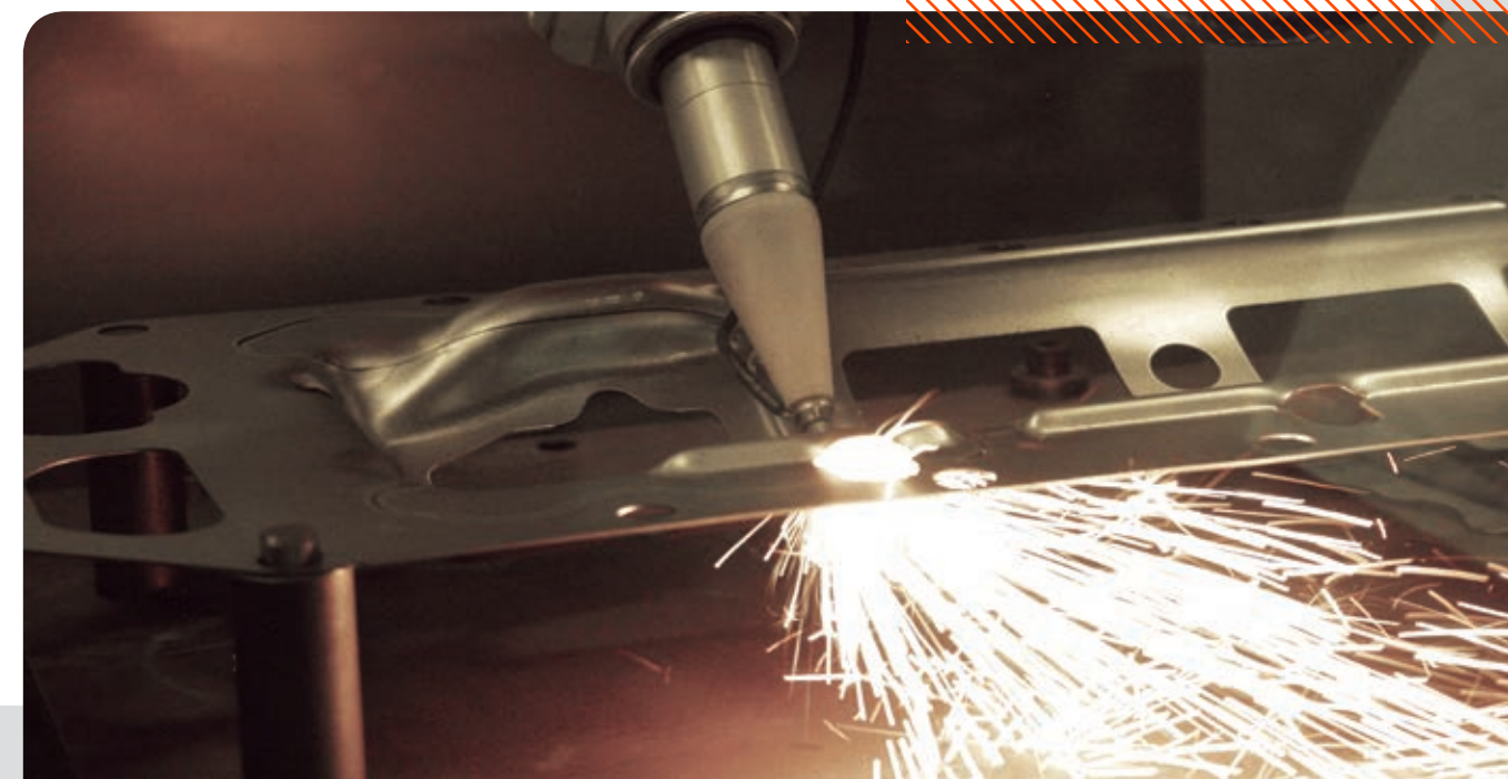
LASERDYNE 430 with BeamDirector cutting shaped holes and contours.
